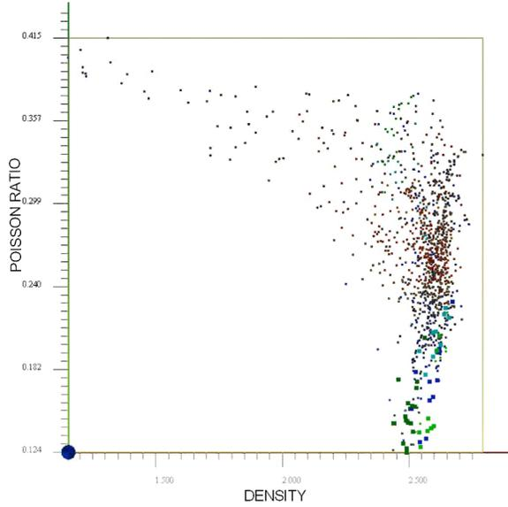
Figure 2. Crossplot of Poisson's ratio ( $\nu$ ) and Density ( $\rho$ ) from well logs. Productive sandstones are shown as larger squares. Most producing zones have Poisson's ratio  $< 0.2$ .
