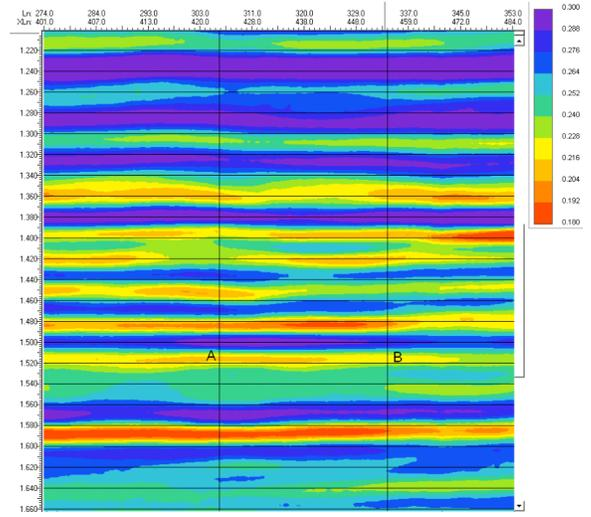
Figure 3. Poisson's ratio section through a productive well (A) and non-productive well (B). Productive interval is at 1.52 sec. Lower Poisson's ratio values are orange and red.
