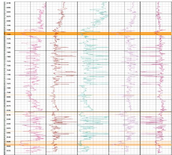
Figure 1. Well logs through formations of interest from left to right are Gamma Ray, P Slowness, S Slowness, Poisson's ratio, and Density. Zones with Poisson's ratio less than 0.2 are highlighted in orange. This well produces from the shallow thick orange zone.
